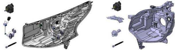
Figure 1. Headlamp assembly components for light housing
