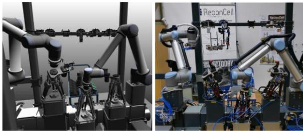
Figure 3. Virtual Testbed (left) of the test workcell (right)
