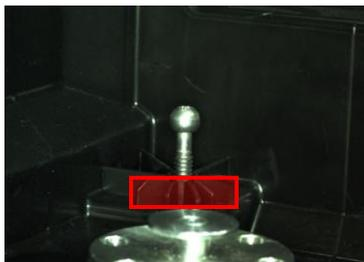
Figure 6. The screw base is selected as ROI and shown red in an overlaid manner.
