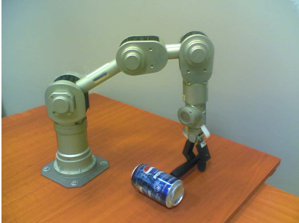
Fig. 2. Side view of the workspace. The robotic arm holds a black plastic tool that is used to push objects on the work surface.
