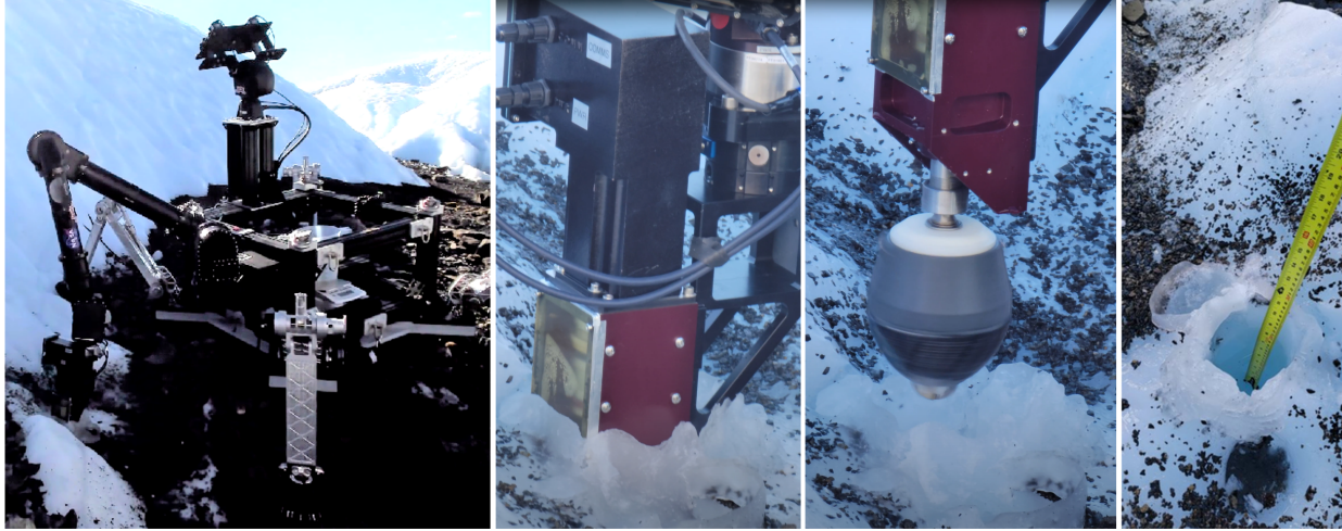
Figure 22: Left: The lander conducting an extended plunge excavation at site C, with the ICEPIC tool pictured deep into the ice on bottom left. Middle: The ICEPIC tool exiting the plunge trench. Right: Measurement of the extended plunge trench which netted 27cm of depth under the original surface.
