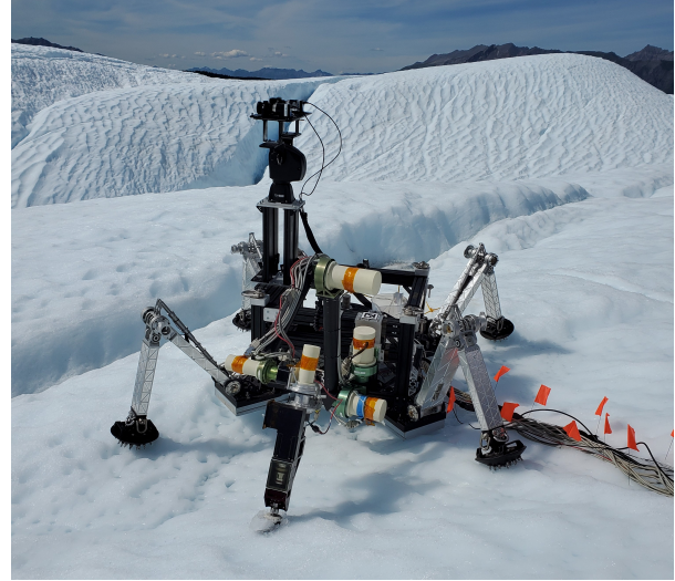
Figure 1: The Europa Lander Field Sampling Campaign (ELFS Camp) system at sampling site A on Matanuska Glacier, AK. Four passively adjustable legs stabilize a central base, atop of which a pan-tilt unit affords pointing of a perception head comprised of a stereo camera pair and LED illuminator. The 5 DoF "Luigi" arm and ICEPIC drilling/sampling tool are seen engaging the ice, while power and compute tethers connect to Ground Support Equipment (GSE) out of view to the right.
