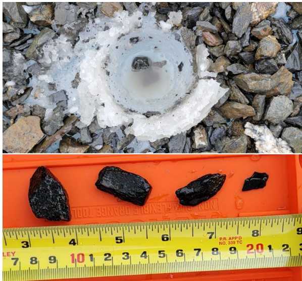
Figure 23: Top: After images of an excavation trench at site C where several rocks fell into the hole during excavation necessitating a manual abort. Bottom: The offending rocks measured for scale.
