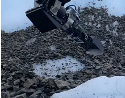
Figure 4: Example scoop interaction with glacier terrain. The top layer is composed of small loose gravel and the lower layer is solid ice. The scoop adapted to the terrain and it removed the top layer to expose the ice beneath for ICEPIC drilling and sampling.
