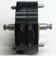
Fig. 2. Two Destaco TP-30 tool adapter modules tightly screwed together.
