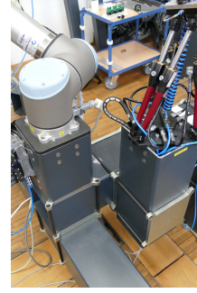
(a) The BoxJoint coupling system holding together steel beams.
