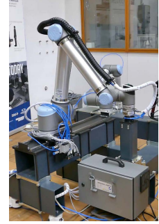
(d) Passive linear axis rail with the robot mounted on it.
