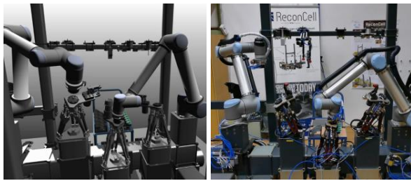
Figure 3. Virtual Testbed (left) of the test workcell (right)
