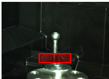
Figure 6. The screw base is selected as ROI and shown red in an overlaid manner.
