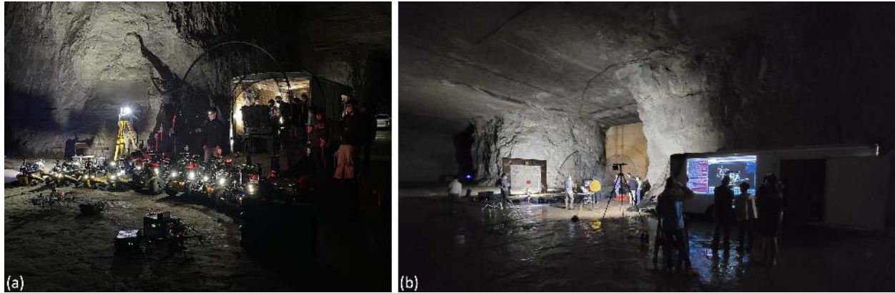
Figure 50: Example test setup for team CoSTAR. a) Full robotic line-up when simultaneously deploying 10 robots (4 spots, 4 huskies and 2 drones) with a single operator in a limestone mine. b) The larger team workspace, including base station projection for team members to observe, and calibration gate to simulate a DARPA course.
