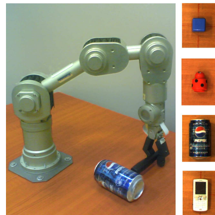
Figure 2: View of the workspace. The robotic arm holds a black plastic tool that is used to push objects on the work surface. Some sample objects are also shown.
