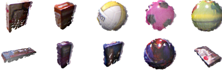
Figure 7.31: Segmented 3-D object point clouds from the KUKA-LWR/Kinect experiment (not to scale).
